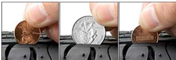
2/32" remaining 4/32" remaining 6/32" remaining
