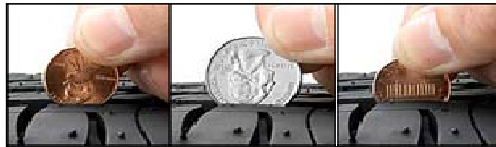
2/32" remaining 4/32" remaining 6/32" remaining
