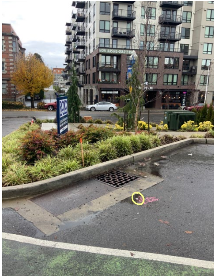
Photograph 5: Pavement Cap Monument "C" offset 4-feet from capped rebar at stake..
