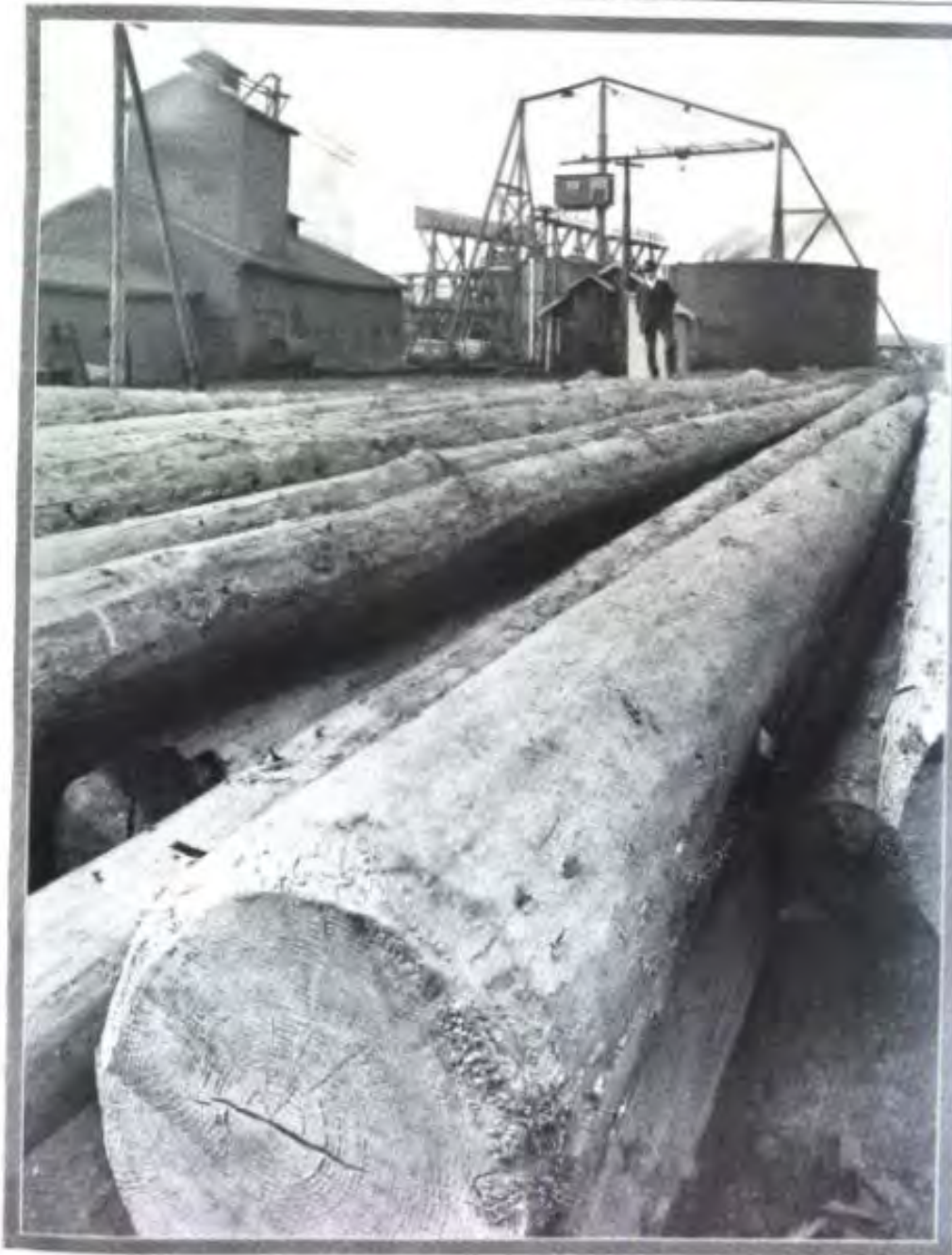
A partial view of the creosoting plant of the St. Paul & Tacoma Lumber Co., at Tacoma, Wash. In the foreground are shown treated piling. Piling, poles, timbers, and railroad ties are the principal creosoted products
