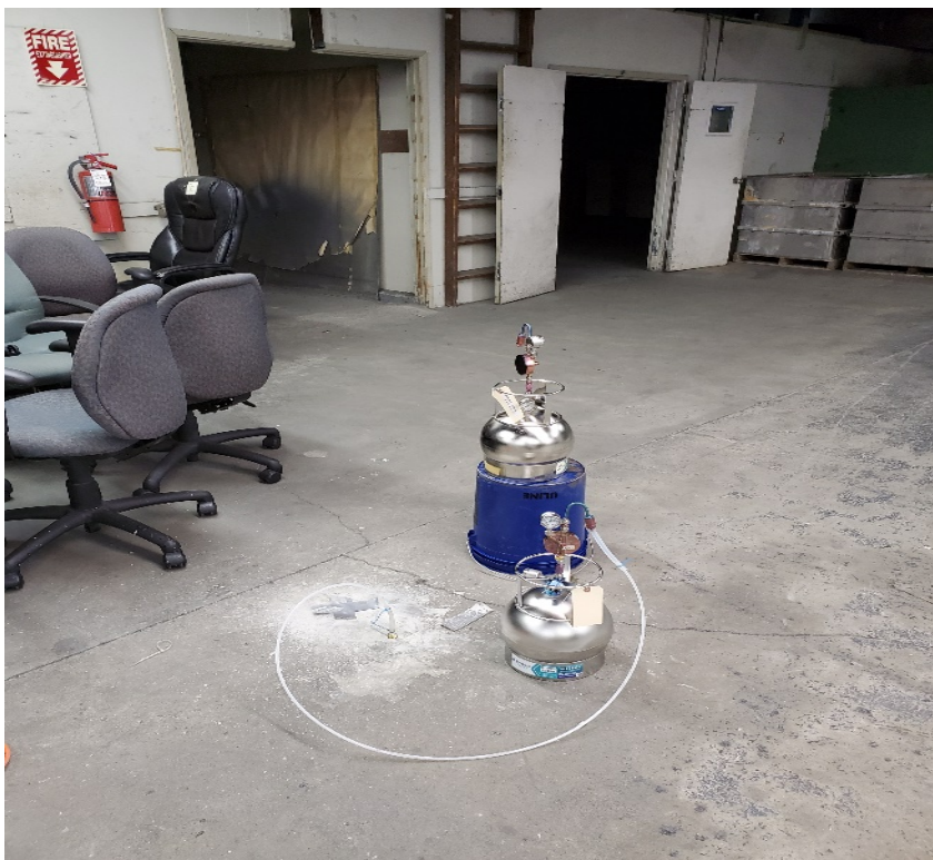
Photograph 1: Date: February 21, 2020 time: 13:18. Sample location and setup of SV-7 and IA-7 in the eastern area of the USM building.
