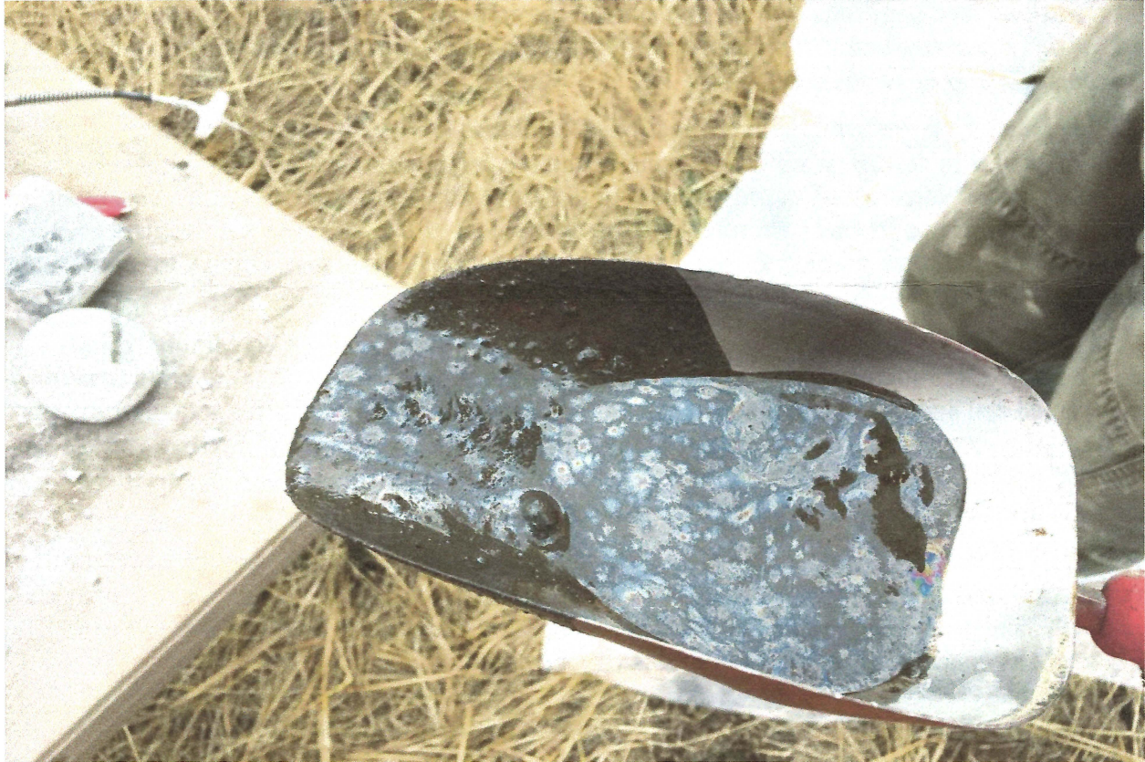
Petroleum sheen in saturated soils from MW-5.
