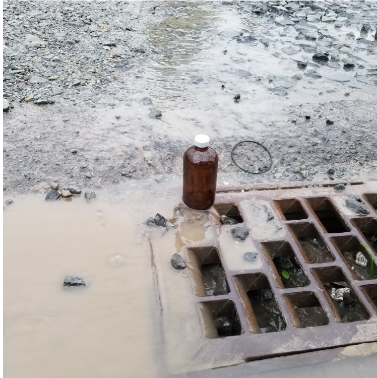
Photograph 1: View of outflow sample jar and sampled 7 th Avenue South stormwater catch basin grate.
