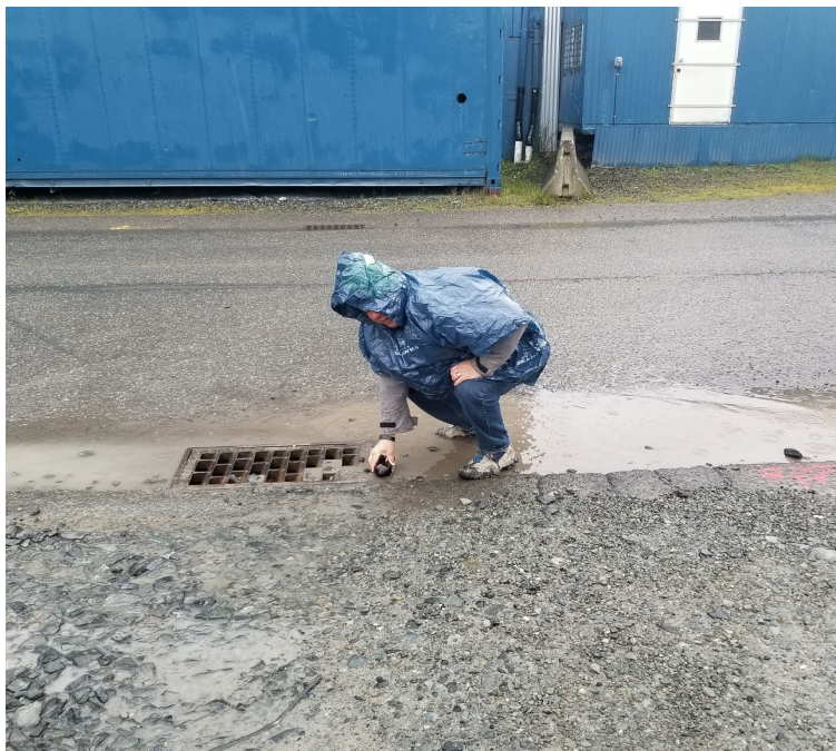
Photograph 2: View of outflow sampling at the 7 th Avenue South stormwater catch basin grate.
