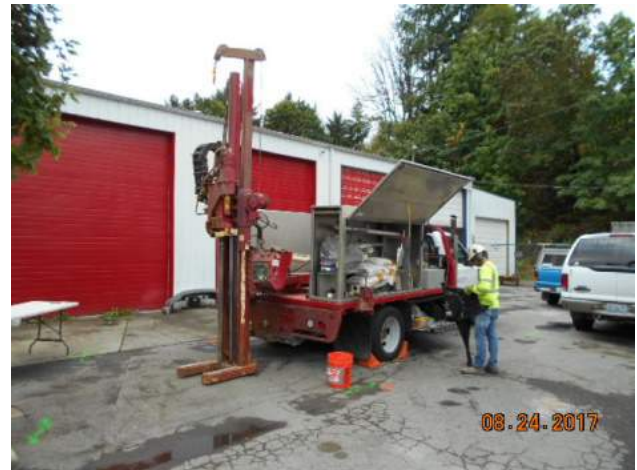
Photograph 2. Installation activities associated with soil boring SB-2, adjacent to the auto repair bays.
