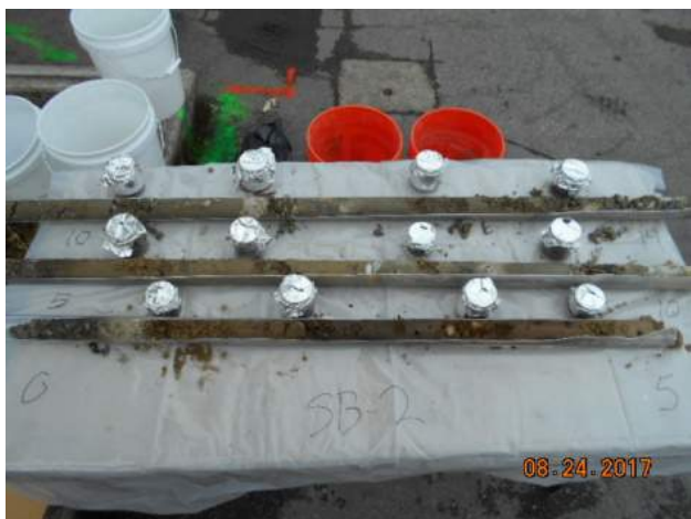
Photograph 9. Typical soil lithology as encountered at soil boring SB-2.
