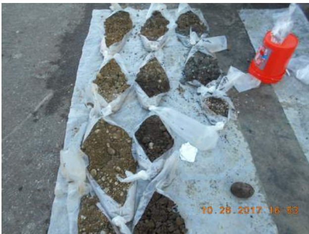
Photograph 3. Soil lithology as encountered at soil borings SB-6, SB-10 and SB-11.
