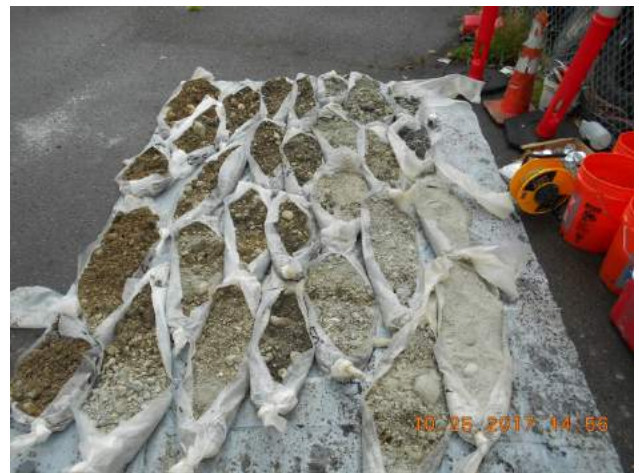
Photograph 4. Typical soil lithology as encountered at soil boring TSB-1.
