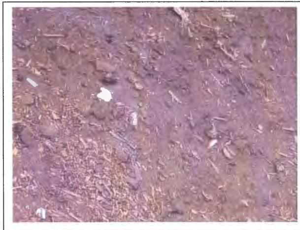
Photo 24. Note the white asbestos containing pipe insulation in the left central portion of the photo in the wood fuel storage area to the south of Boiler 4.
