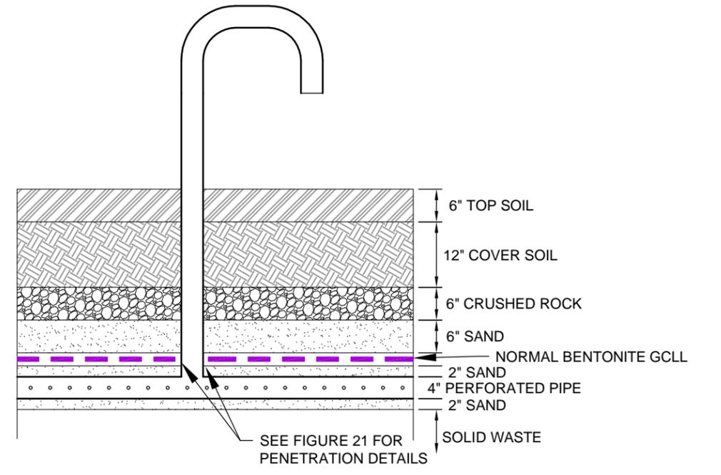
2 PASSIVE LANDFILL GAS VENT DETAIL
