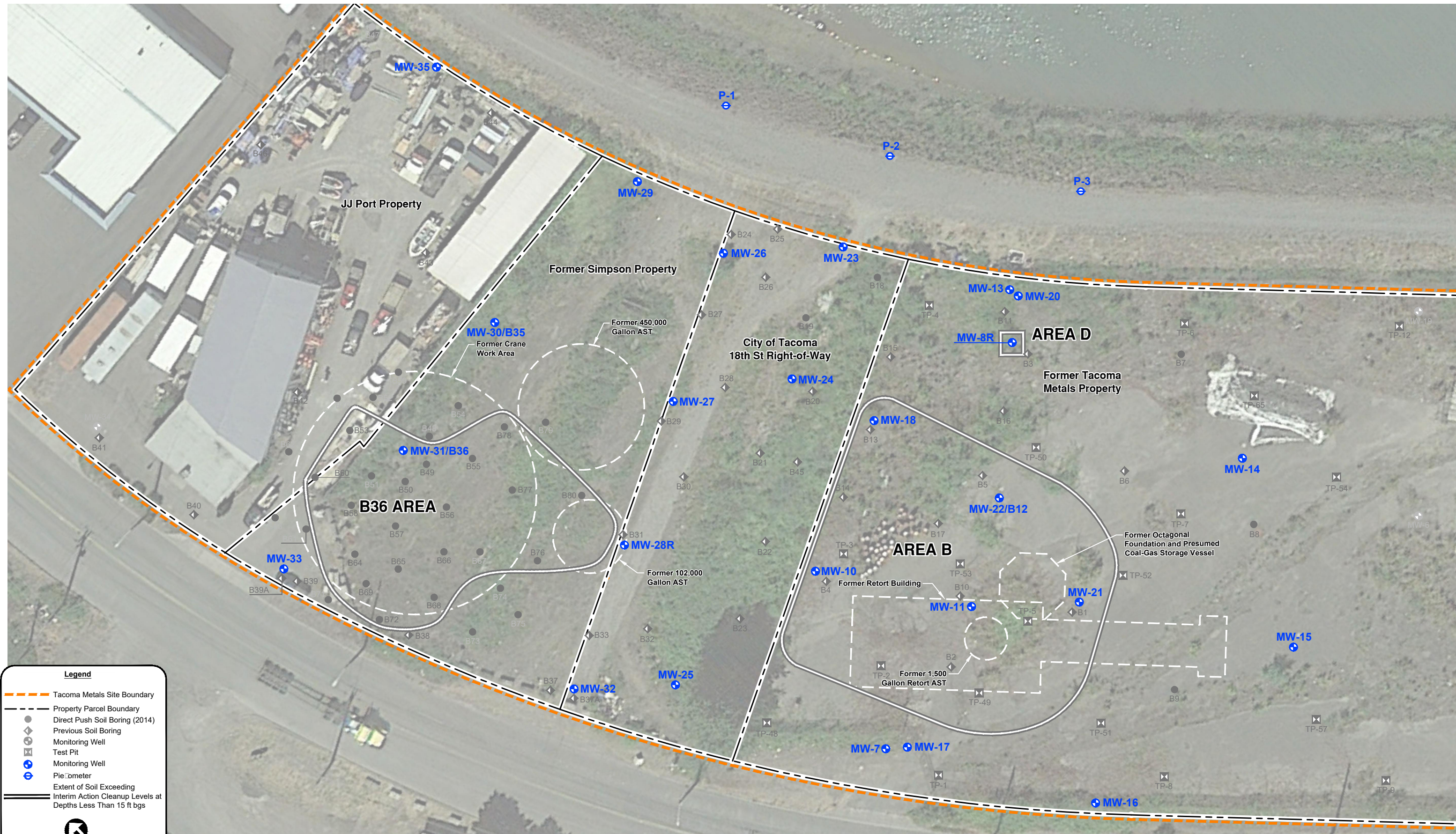
Figure E-2 Supplemental Investigation Groundwater Sampling Locations B36 Area, Area B, and Area D
