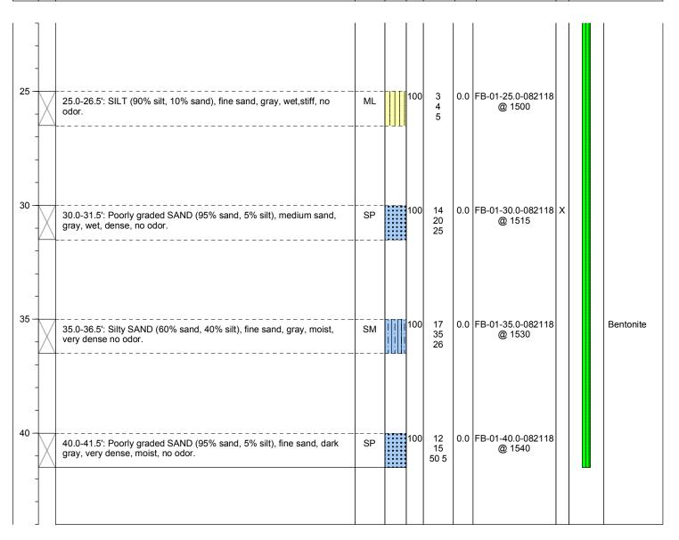
**Well Construction Information** Ground Surface Elevation (ft): NA Monument Type: NA Filter Pack: NA Casing Diameter (inches): Top of Casing Elevation (ft): NA NA Surface Seal: Concrete Surveyed Location: Screen Slot Size (inches): NA Annular Seal: X:NA NA Screened Interval (ft bgs): NA **Boring Abandonment:** Bentonite Y: NA
