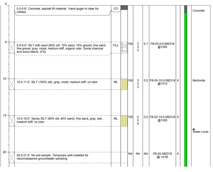
**Well Construction Information** Monument Type: NA Filter Pack: NA NA Casing Diameter (inches): Surface Seal: Concrete Surveyed Location: Screen Slot Size (inches): NA Annular Seal: NA Screened Interval (ft bgs): NA **Boring Abandonment:** Bentonite
