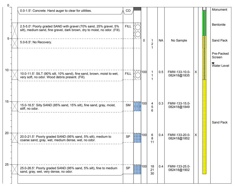
Monument Type: Flush Mount Casing Diameter (inches): 10 Screen Slot Size (inches): 0.01 Screened Interval (ft bgs): 6.5 - 11.5 **Well Construction Information**
