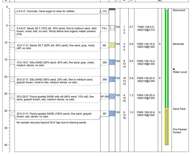
Monument Type: Flush Mount Casing Diameter (inches): 10 Screen Slot Size (inches): 0.010 Screened Interval (ft bgs): 30.0-40.0
