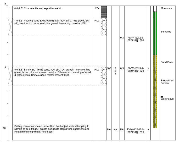
Monument Type: Flush Mount Casing Diameter (inches): 10 Screen Slot Size (inches): 0.010 Screened Interval (ft bgs): 5.0-10.0 **Well Construction Information**
