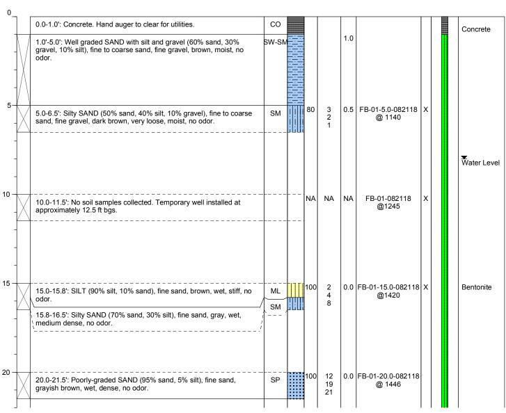
**Well Construction Information** Ground Surface Elevation (ft): NA Monument Type: NA Filter Pack: NA Top of Casing Elevation (ft): NA NA Casing Diameter (inches): Surface Seal: Concrete Surveyed Location: Screen Slot Size (inches): NA **Annular Seal:** X:NA NA Screened Interval (ft bgs): NA **Boring Abandonment: Bentonite** Y: NA
