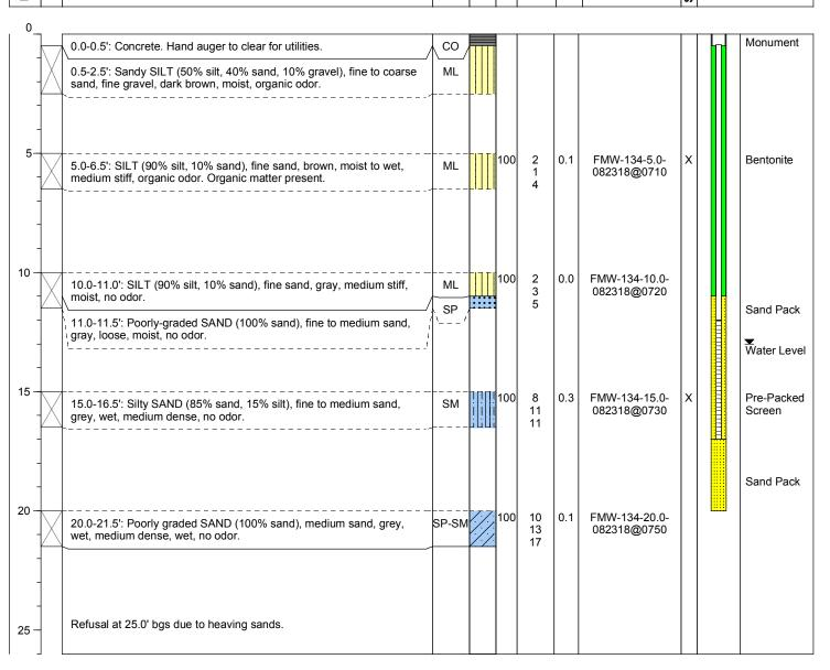
Monument Type: Flush Mount Casing Diameter (inches): 10 Screen Slot Size (inches): 0.010 Screened Interval (ft bgs): 12.0-17.0
