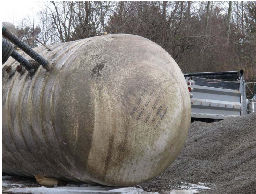
9. Labeled end of intact UST. Label reads "MODEL DWT TYPE II / DOUBLE WALL TANK / 12000 GALLONS / UL 38003 / LAFD 40-90-1"
