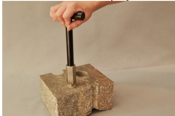
Figure 7. Removing the VAPOR PIN®
