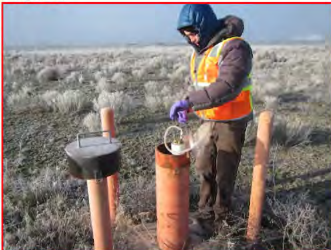
Figures 12 and 13: Jonathan Moen inspects airport well 91AW16 and measures static water level. The team was unaware the well contained a dedicated bladder pump. This well will be sampled in February 2015.
