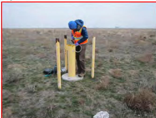
Figure 22: Attaching tubing, air lines, and cables required to sample well 99BW18.
