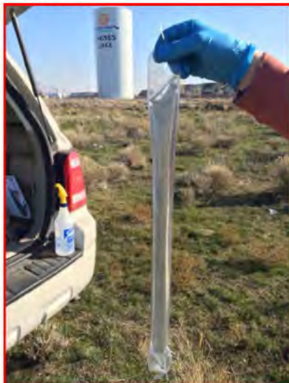
Figure 28: A typical passive diffusion bag recovered from well 04BW05 prior to being cut open for immediate VOC sample collection. A new PDB was then reinstalled in the well.
