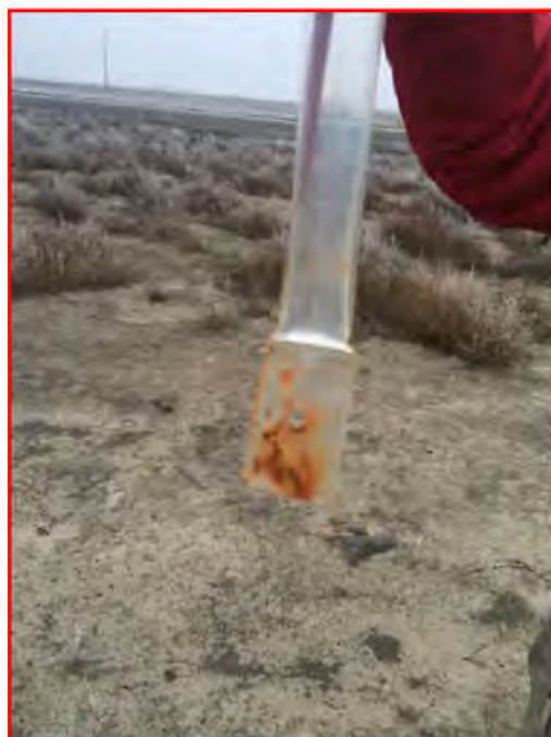
Figures 30 and 31: Rust residue on suspension line and bottom of PDB from steel well casing at well 14EX03.
