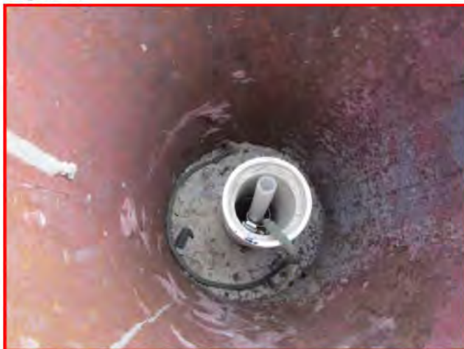
Figure 18: Inside casing view of monitoring well 91AW01 found to contain sample tubing for a submersible pump presumably used by contractors.
