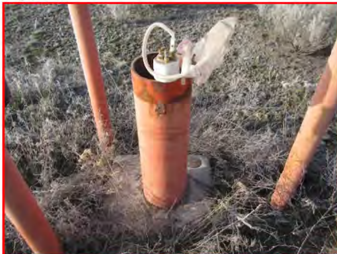
Figures 12 and 13: Jonathan Moen inspects airport well 91AW16 and measures static water level. The team was unaware the well contained a dedicated bladder pump. This well will be sampled in February 2015.
