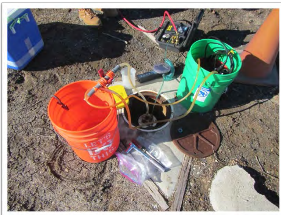
(160223-99BW10-1) Purging bladder pump well 99BW10.
