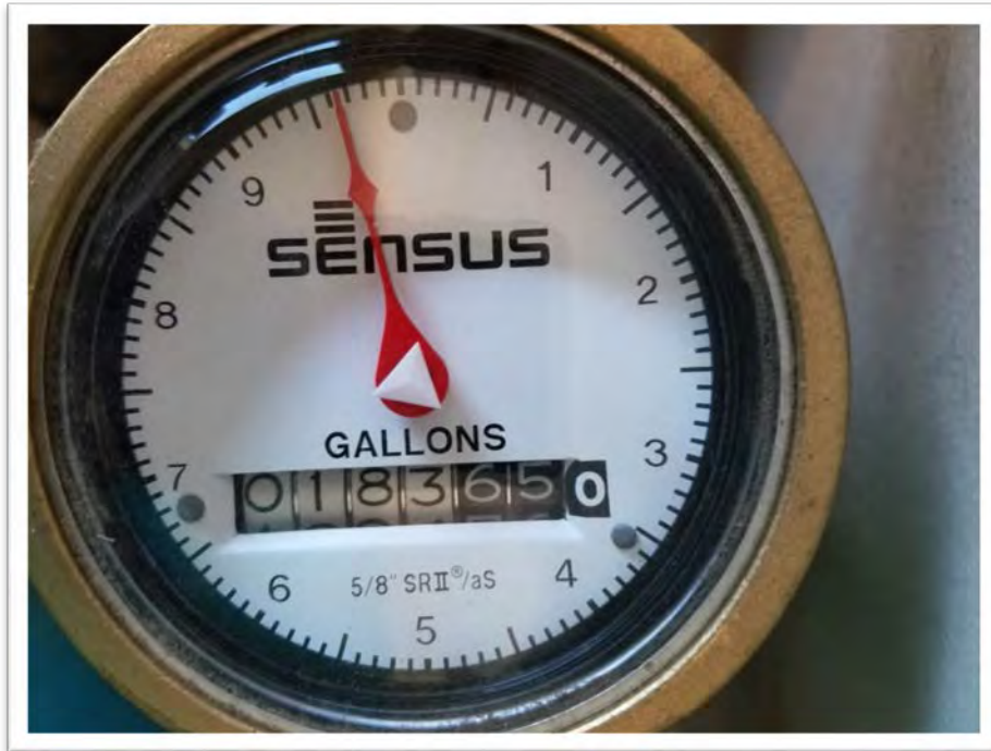
(20161115-151928) Detail photo of totalizer gauge showing 183,659.5 gallons have passed through the gauge since it was installed.
