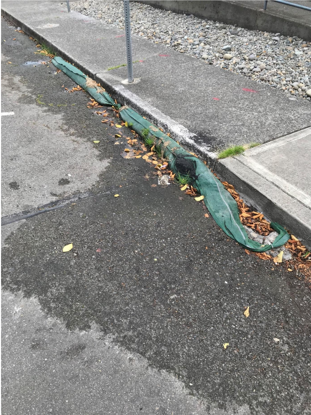
Figure 1: Photo of seep socks taken August 11, 2020. Note seep water extending into street and poor condition of socks including ripped outer cover on seep sock and exposed granular activated carbon.
