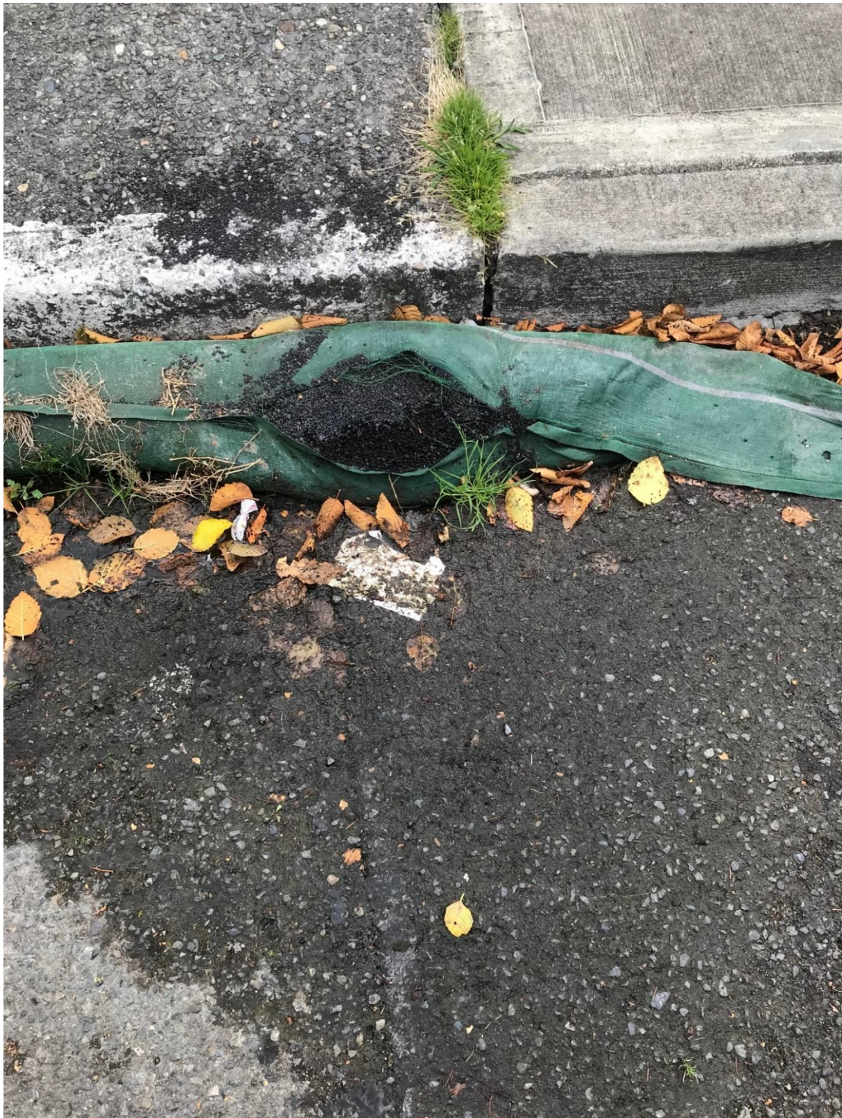
Figure 2: Close-up of ripped outer covering of sock and exposed granular activated carbon.
