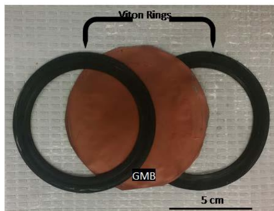
Figure 2: Membrane and Viton Rings
