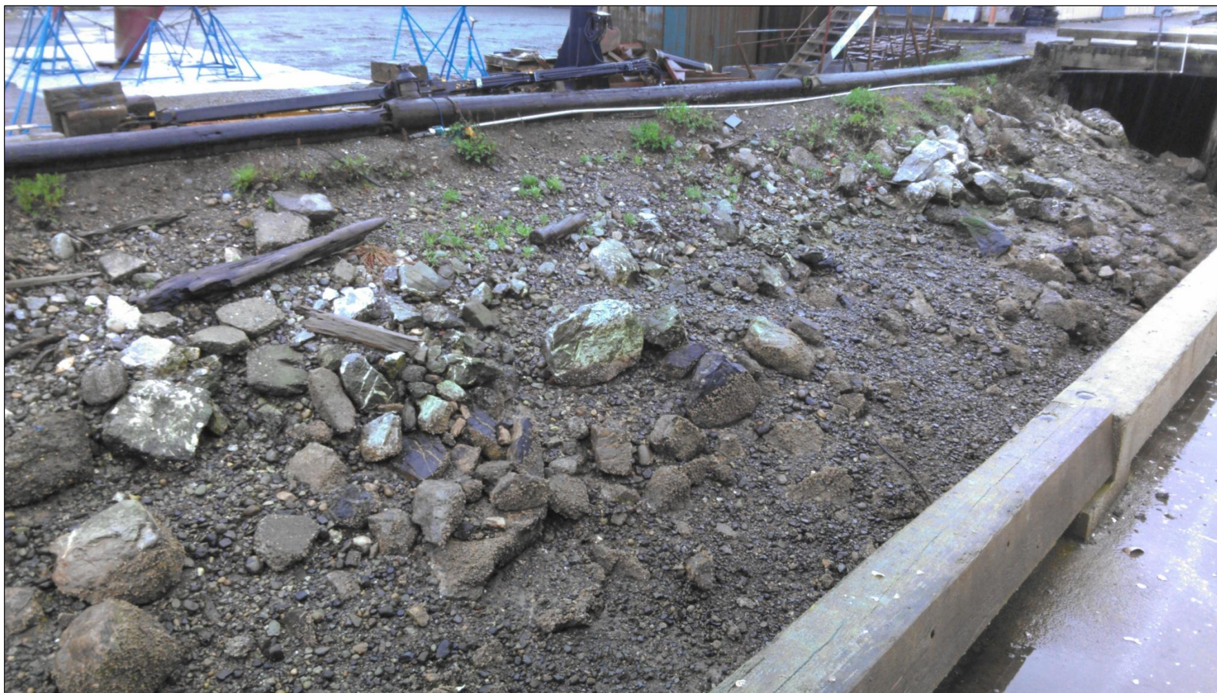
7. Shoreline conditions at sediment sample location WM-SG-16: mostly rock slope with some gravel and sedimentation. At sample location WM-SG-28 (background, right), insufficient sediment was present on the rock to collect a sample for analysis.
