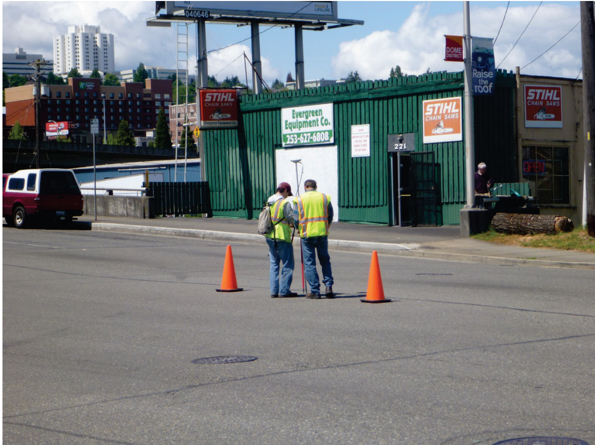
Figure 2-3 - 2014 Survey RTK GPS Vertical Control Location – Benchmark 1823/3547
