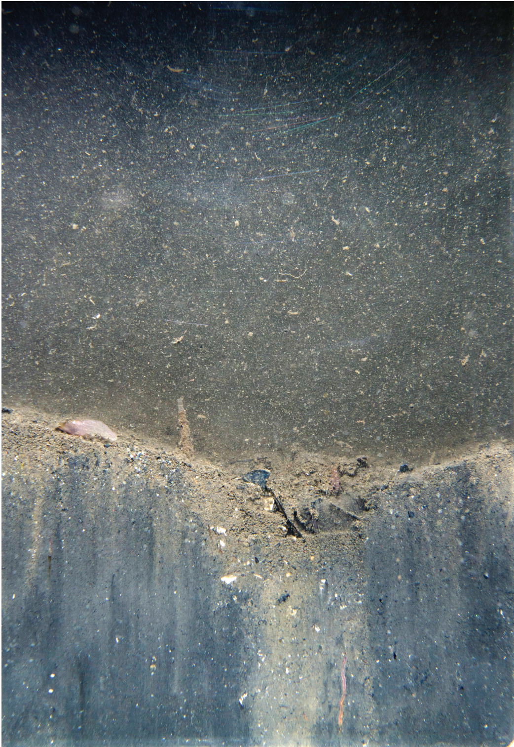
Figure 8: The large surface boundary roughness values measured at Station Y10-S15-I were due to biogenic burrow openings or mounds; note the large polychaete tube sticking above the sediment surface to the left of the burrow opening. Scale: width of profile image =14.5 cm.
