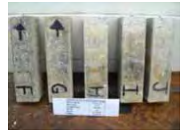
Hycrete prisms after 18 months of exposure
