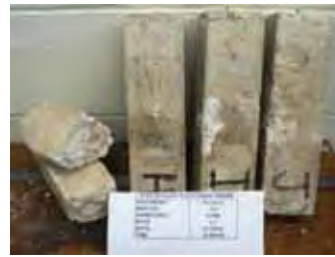
Control prisms after 18 months of exposure
