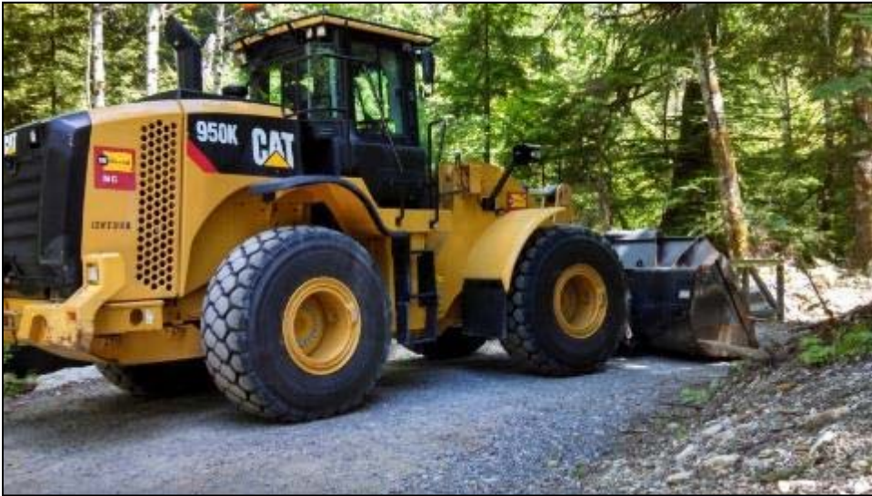
Photograph 20. Cleaned, weed-free CAT 950K Loader upon arrival to the Site (CES 6/15/2015).
