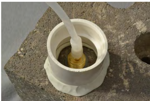
Figure 6. Water dam used for leak detection
