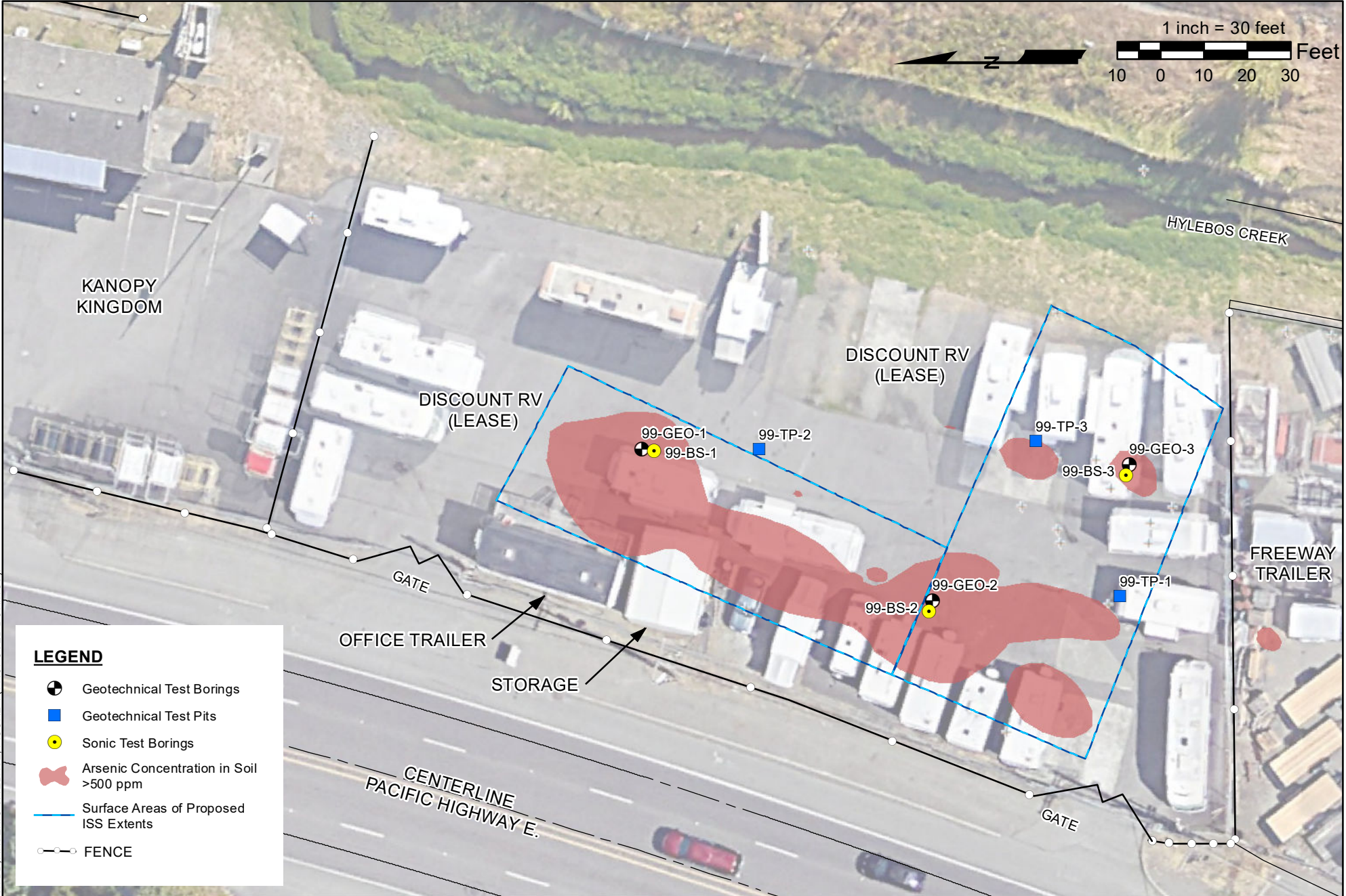
Figure 5 Proposed Boring Location Plan
