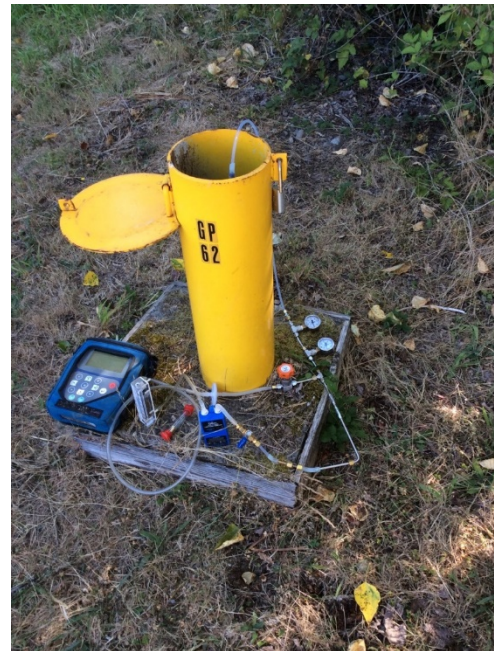
Photograph 4. Purging prior to sampling at GP-62.
