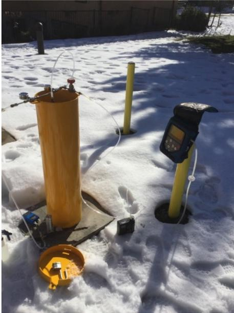
Photograph 1: High-flow purge sample train set up at GP-63C.
