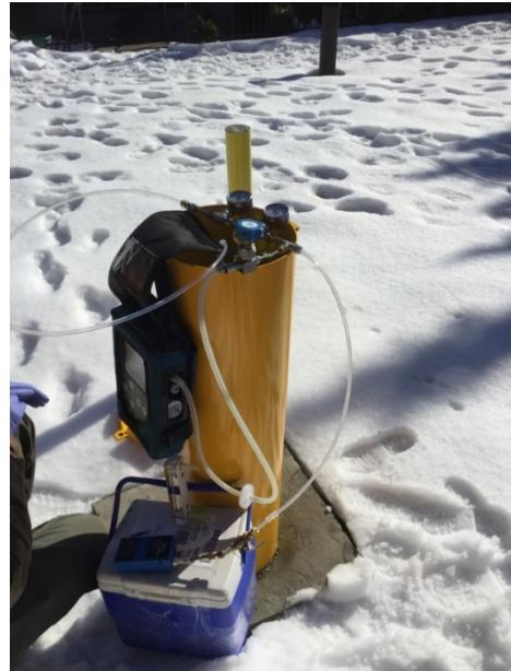
Photograph 2: Aspect staff monitor methane readings during the purge of GP-63B.
