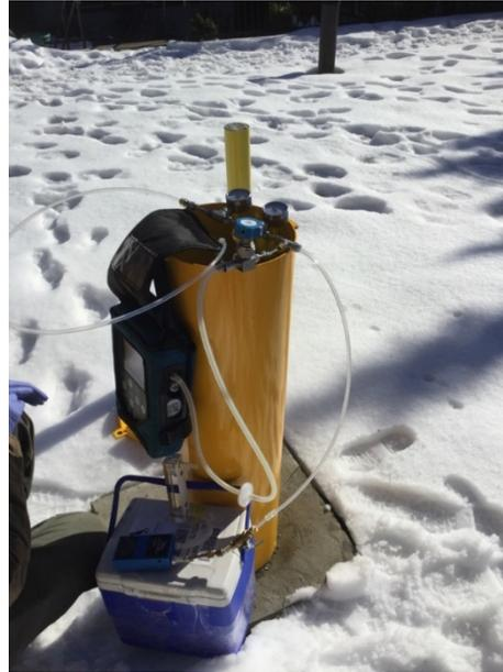
Photograph 2: Aspect staff monitor methane readings during the purge of GP-63B.
