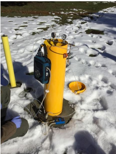
Photograph 3: Aspect staff monitor methane readings during the purge of GP-64C.
