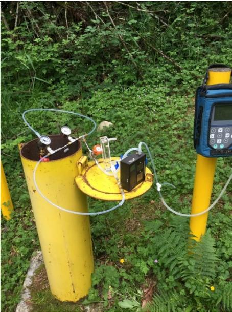
Photograph 3: Aspect staff monitor methane readings during the purge of MW-102.
