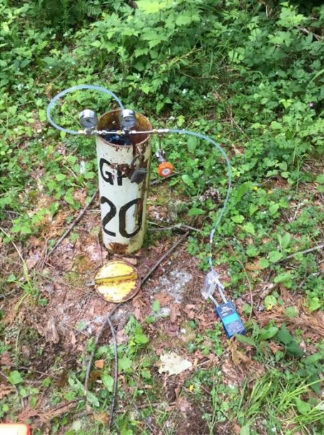
Photograph 1: High-flow purge sample train set up at GP-20A/C.
