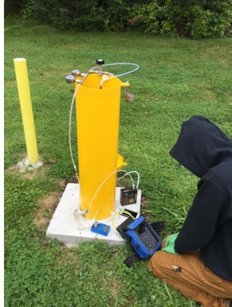
Photograph 2: Aspect staff monitor methane readings during the purge of GP-63B/C.
