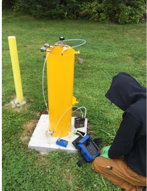
Photograph 2: Aspect staff monitor methane readings during the purge of GP-63B/C.
