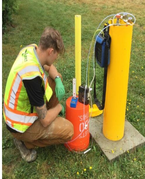
Photograph 2: Aspect staff monitor methane readings during the purge of GP-64B/C.
