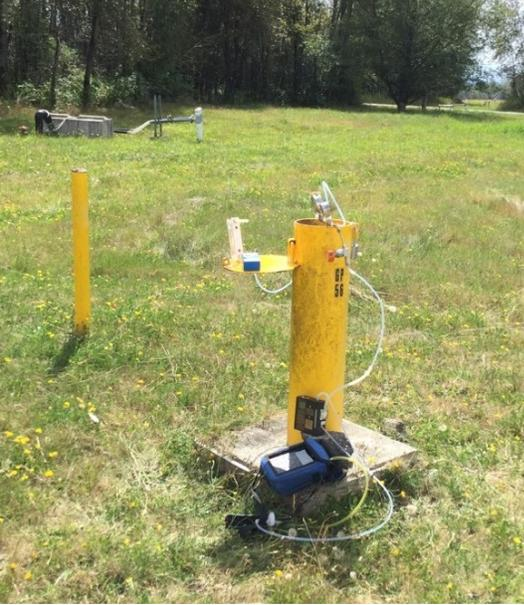
Photograph 1: High-flow purge sample train set up at GP-56.
