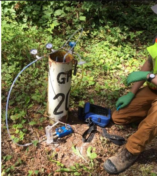
Photograph 3: Aspect staff monitor methane readings during the purge of GP-20A/C.
