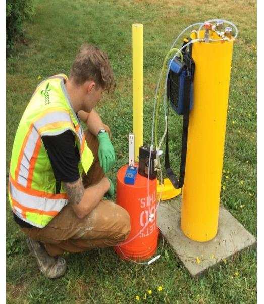
A person wearing a high-visibility vest and green gloves is kneeling on the grass next to a yellow cylinder. They are holding a blue handheld methane detector and looking at its screen. A red drum labeled 'CETCO' is nearby, along with other equipment. |
