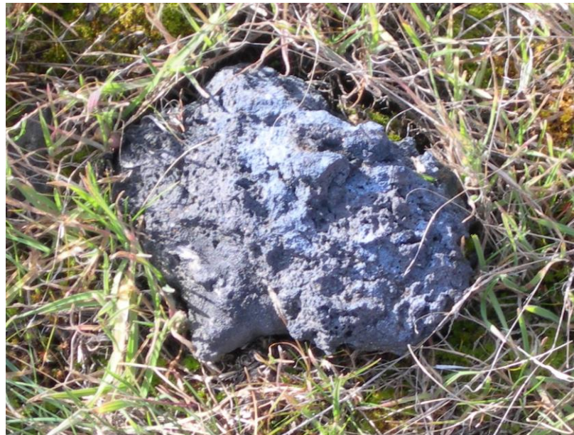
Figure 9 – SPL with recrystallization and vugs
