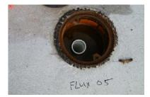
5) Attach retrieval rope (or wires) to the top of each PFM using a carabineer connector.
