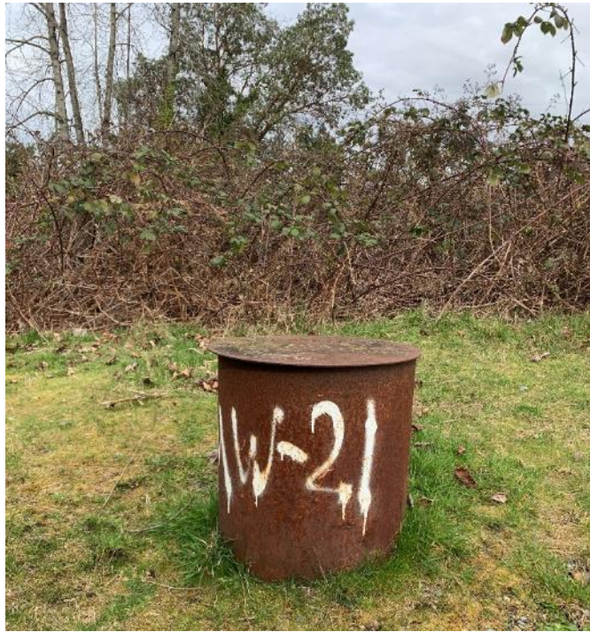
Monitoring well MW-21
