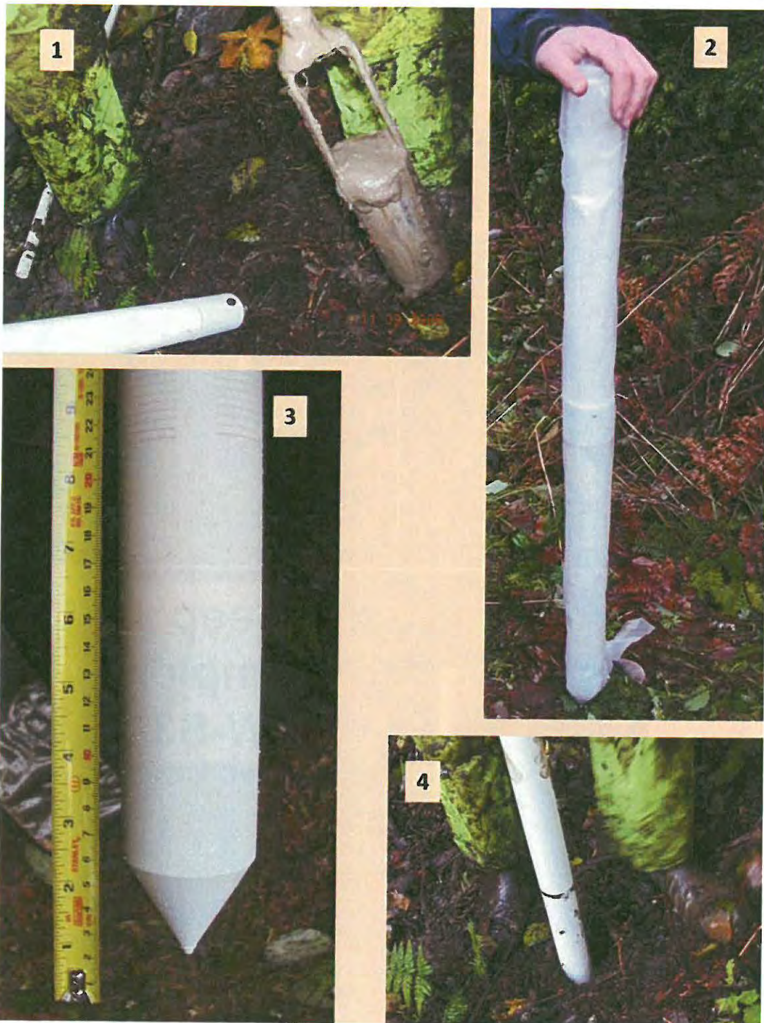
(1) Borehole was hand augered through soil and into underlying sediments (2) Sampler was constructed of clean 2-inch Sch. 40 PVC with 0.010-slot screen (3) Bottom PVC Monopoint; 0.010-inch slots visible at top of picture (4) Inserting seepage sampler into borehole.
