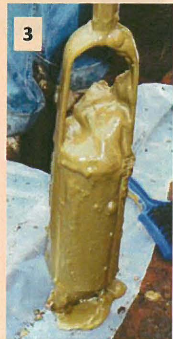
(1) Hand augering through platform access hole (2) Removing coring sediments (3) Saturated sediments in auger bit (4) Driller using soil sampler
