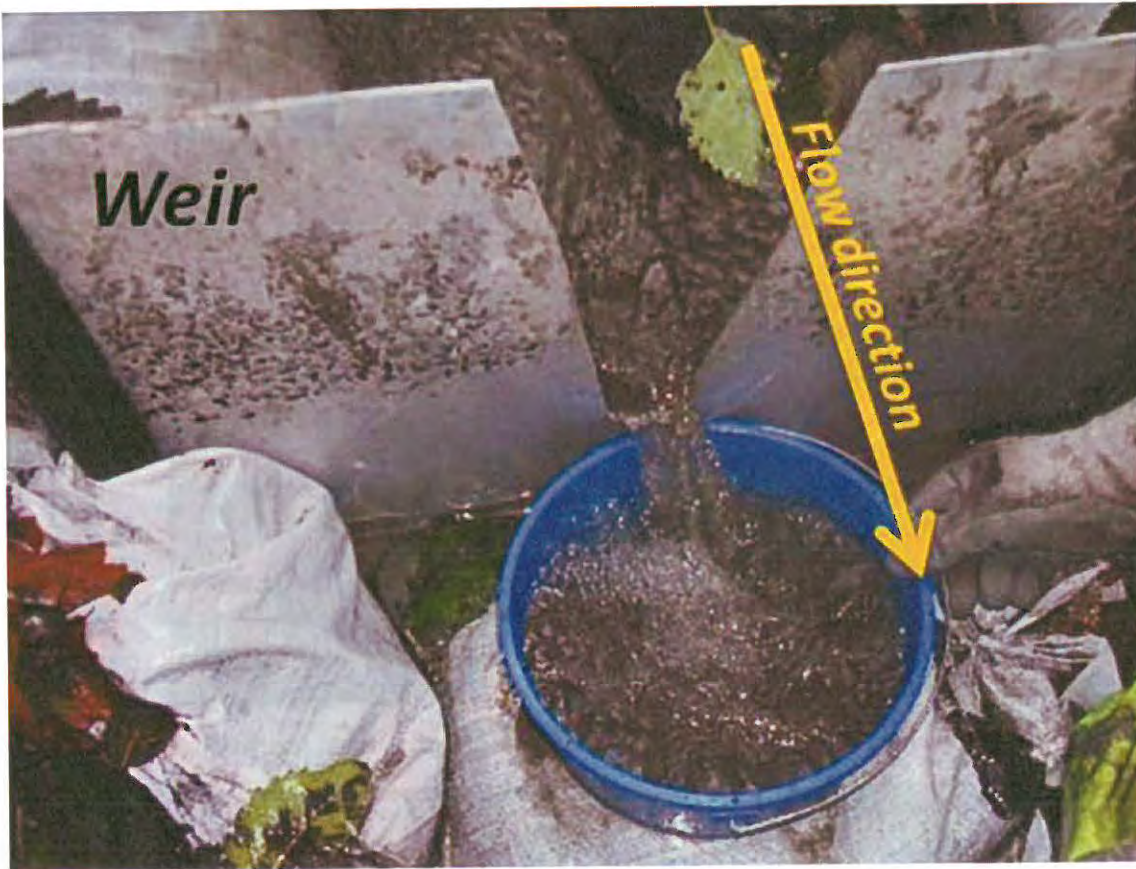
The above photo shows a catch with a lot of sediment (Sed) and splashing (S).
