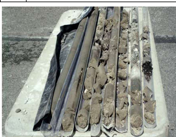
Photo #10: Soil profile collected from boring location B-1. Surface top right, total depth at bottom left. Profile shows the subsurface was predominantly gray, stiff, sandy silt to 22 feet bgs.
