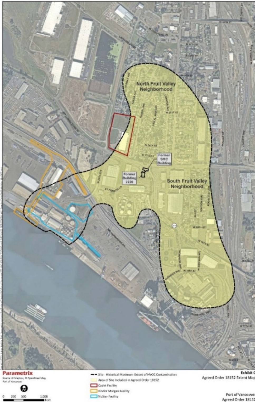
Figure 2. The black dashed line outlines the maximum extent of the solvent plume. The yellow shaded area is the area considered in draft AO DE 18152.
