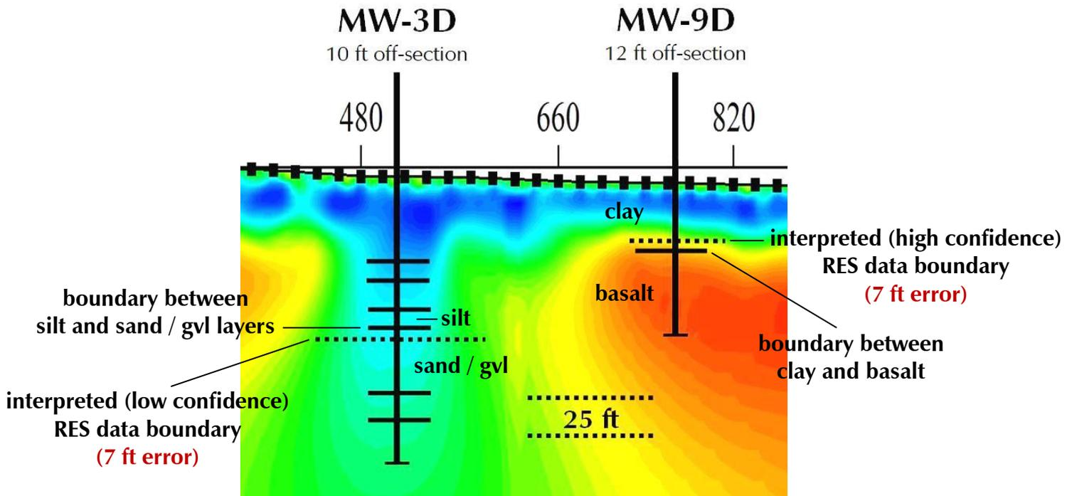
**Figure 1** – Approximate vertical resolution (ie, accuracy) of RES/IP data, as determined from an empirical analysis of the correlation of the data with boring log information.
