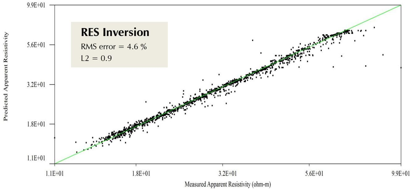
Iteration = 3   RMS = 4.56%   L2 = 0.88   Electrode Spacing = 20 ft
