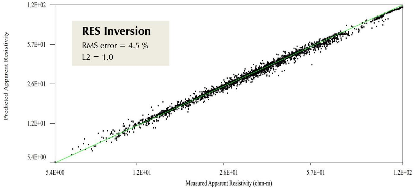
Iteration = 3   RMS = 4.45%   L2 = 0.99   Electrode Spacing = 20 ft
