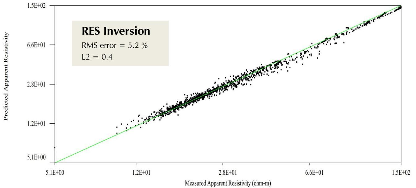
Iteration = 2 RMS = 5.20% L2 = 0.43 Electrode Spacing = 20 ft
