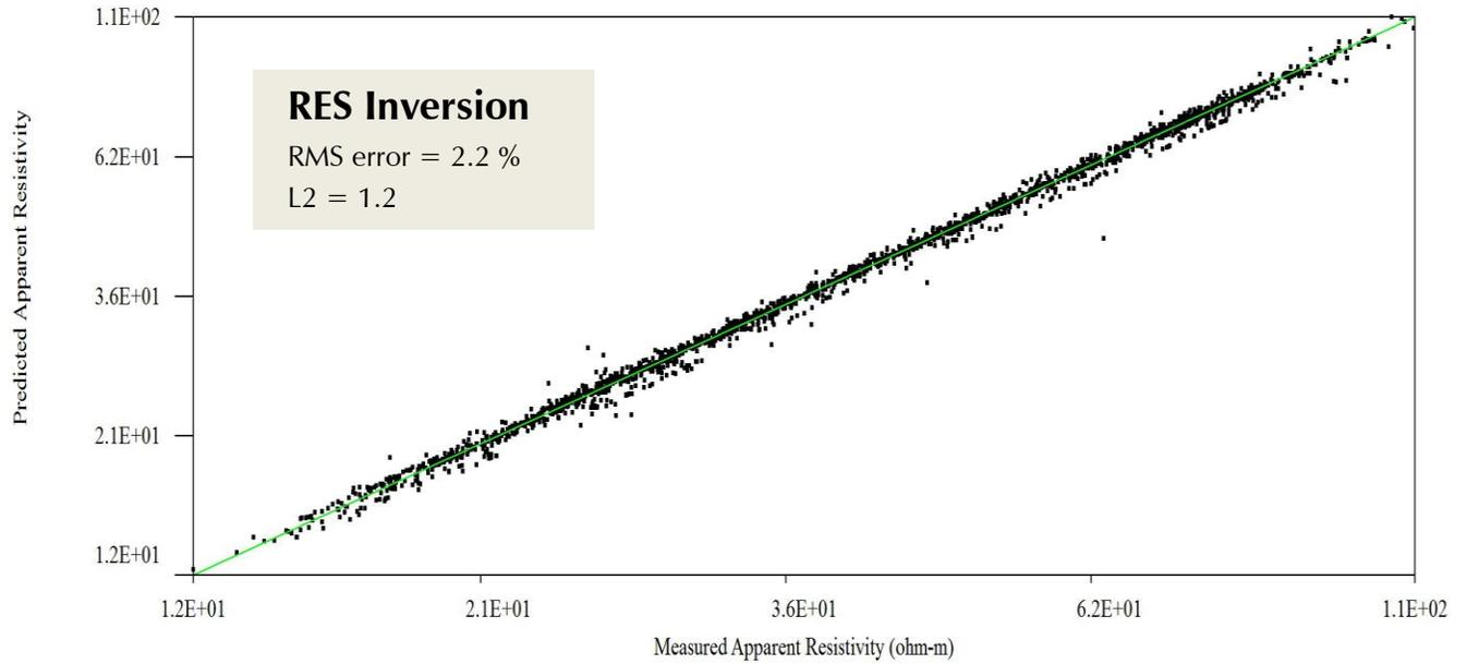
Iteration = 10 RMS = 2.16% L2 = 1.17 Electrode Spacing = 20 ft
