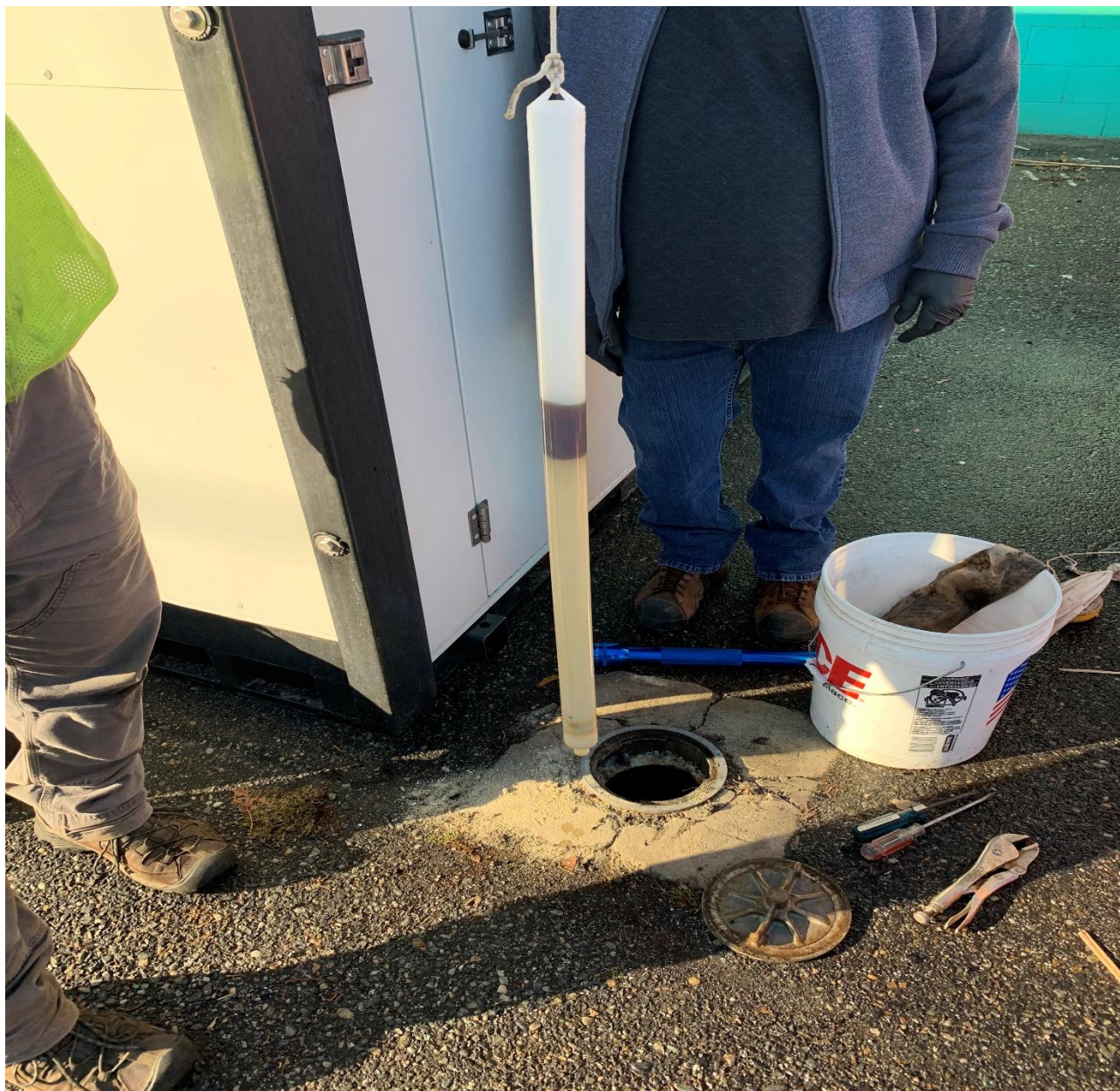
Photograph 4 – Light, non-aqueous phase liquid (LNAPL) removed from monitoring well MW-2 on November 11, 2020 (facing west).
