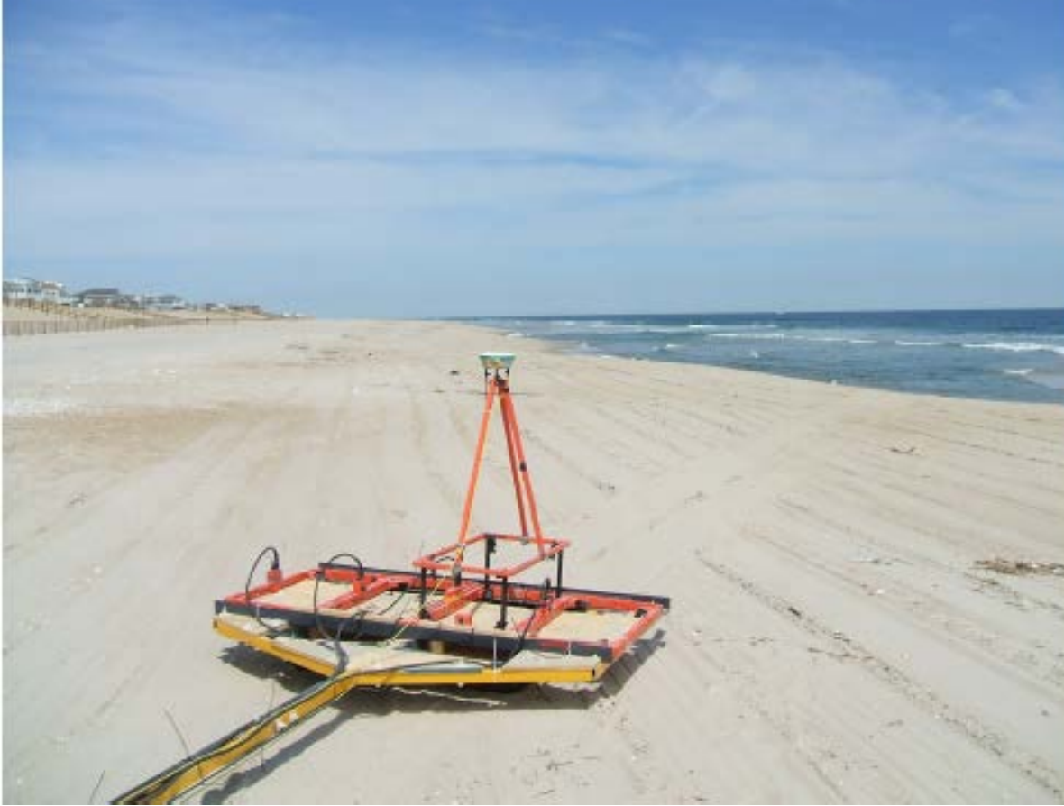
Photograph 1: Four coil configuration of the EM61-MK2 Towed-Array
