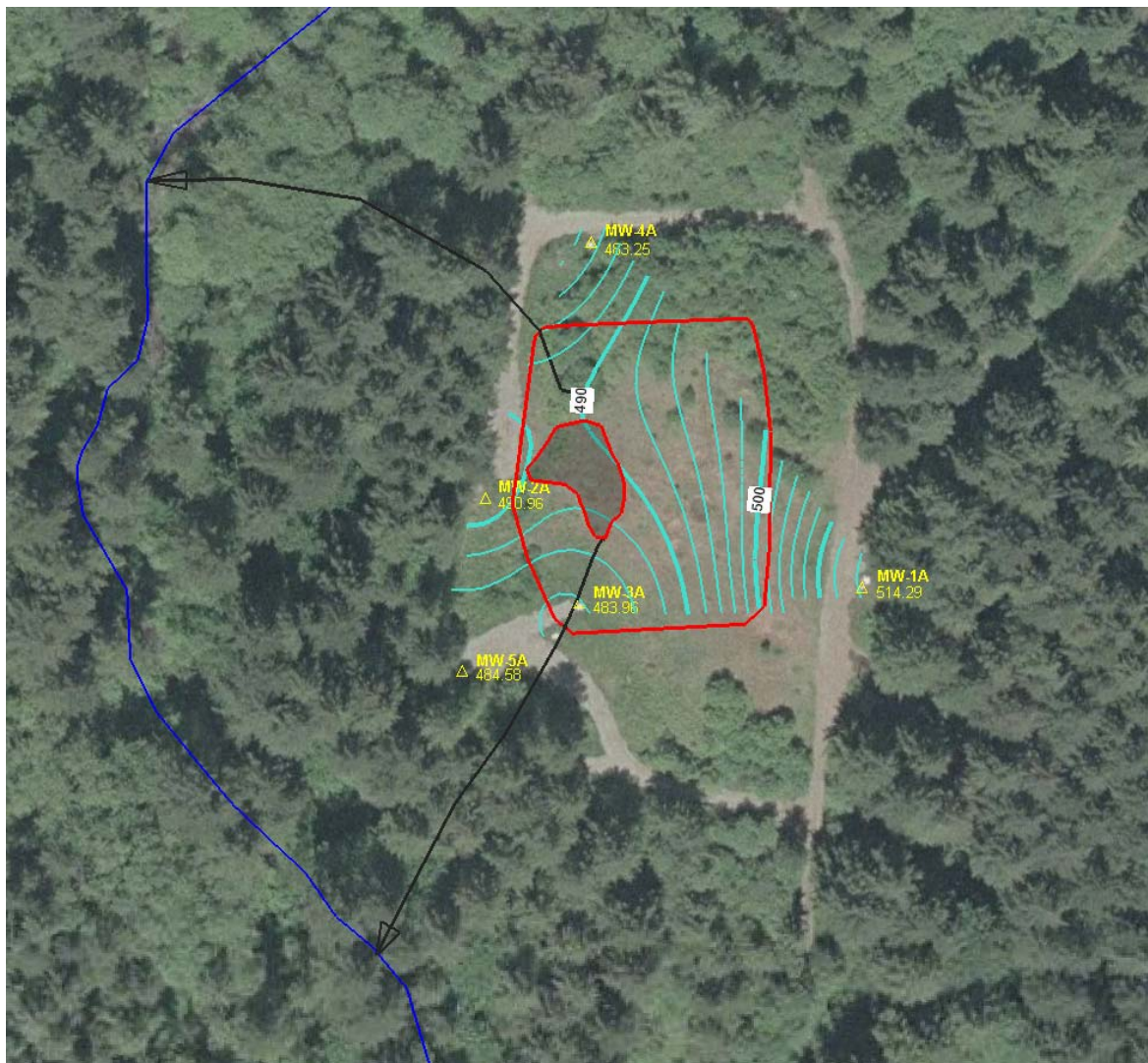
Figure 3.9 – Typical shallow groundwater elevation contours. Black arrows indicate flow lines from area of highest perchlorate concentration in soil.
