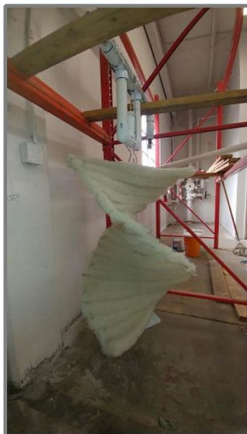
Frame 9-1: Interior design of Air Stripper 2. A brass nozzle sprays water up and the resultant mist falls through the helical media below. (12/1/2018)
