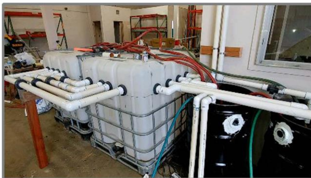
Frame 11-4: To handle the increased amount of water being pumped by the jet pumps, two additional 250 gallon sediment tanks along with 2 drums to transfer water to the rest of the system were added. (3/24/2019)
