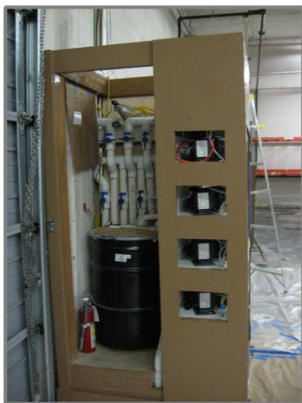
Frame 2-3: Cabinet to house paristaltic pumps, settling drum VES valves and H2O filters. (1/27/2010)
