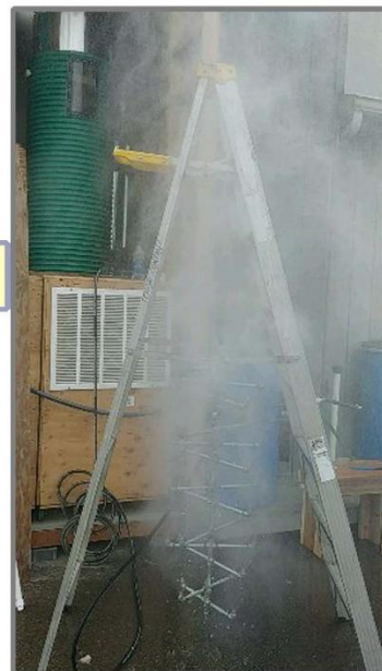
Frame 9-2: Demonstration of Air Stripper 3's spray nozzle system. (4/30/2018)
