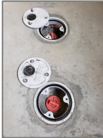
Frame 19-2: Each monument has a locking cap atop the access point as shown. (2/24/2020)
