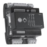
The IO 112 is a measuring module and a 1-channel protection unit for use in connection with the MP 204 motor protection unit. The module can be used for protection of pump against other factors than the electrical conditions, for instance dry-running. It can also be used as a stand-alone protection module.
