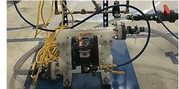
Figure 4. AODD filter press pump.
