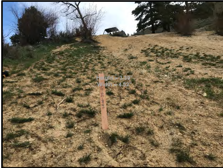
Photograph 35. View northeast toward downslope sample location SR06-DS-07. Note the eroded surficial material. XRF readings identified total arsenic as high as 675 ppm.
