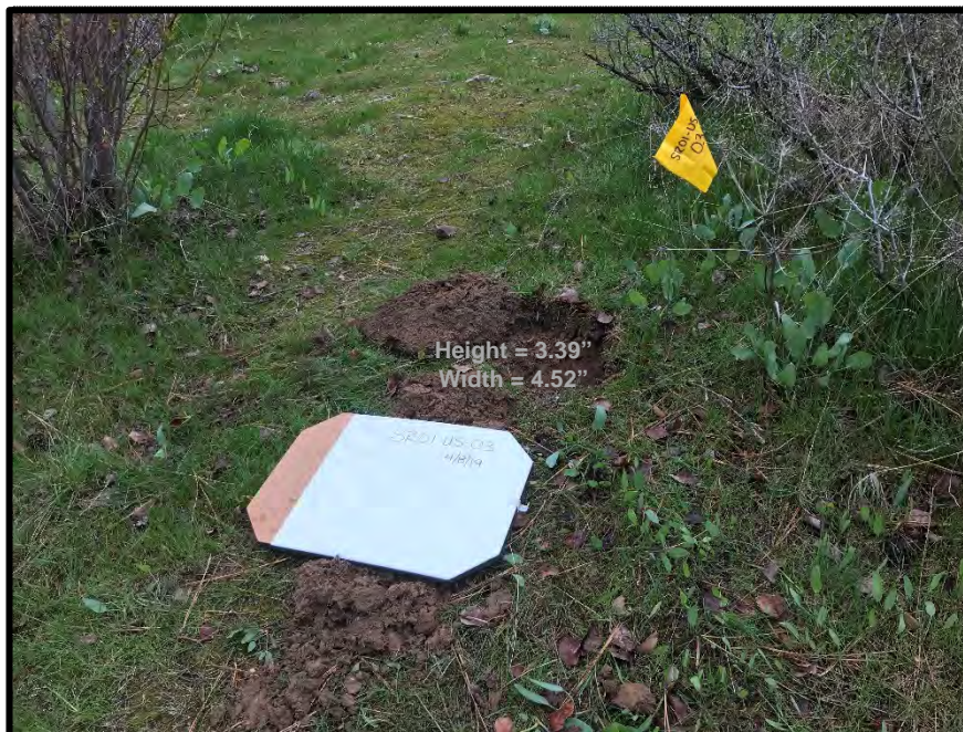
Photograph 6. Upslope sample location SR01-US-03. Total arsenic ranged from 71-73 ppm at this location with the XRF.
