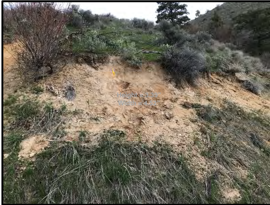
Photograph 33. Looking north toward upslope sample location SR06-US-16. Note the eroded surficial material. XRF readings identified total arsenic as high as 301 ppm.
