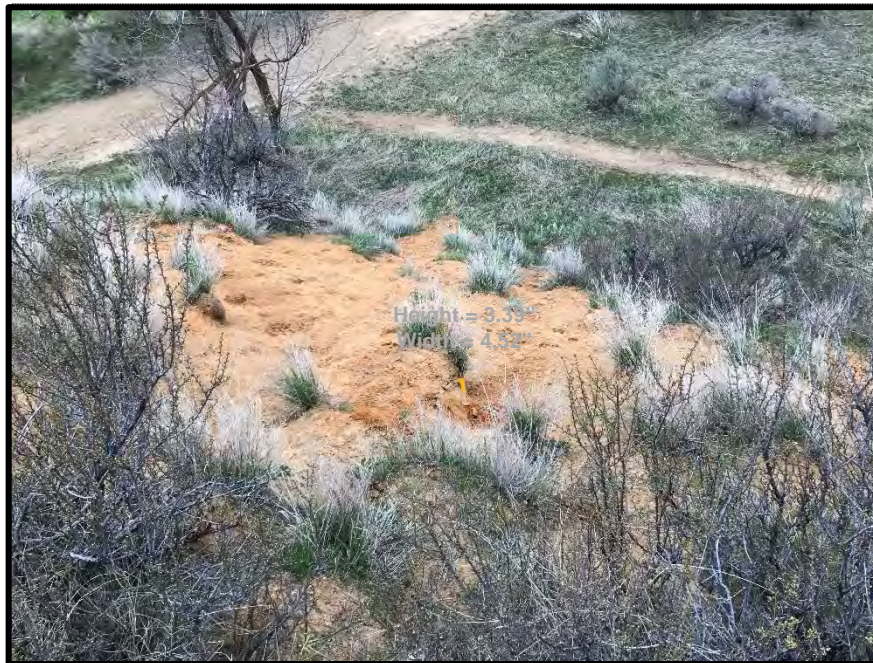
Photograph 32. View north toward upslope sample location SR06-US-07. Note the eroded surficial material. XRF readings in the location were as high as 728 ppm for total arsenic.
