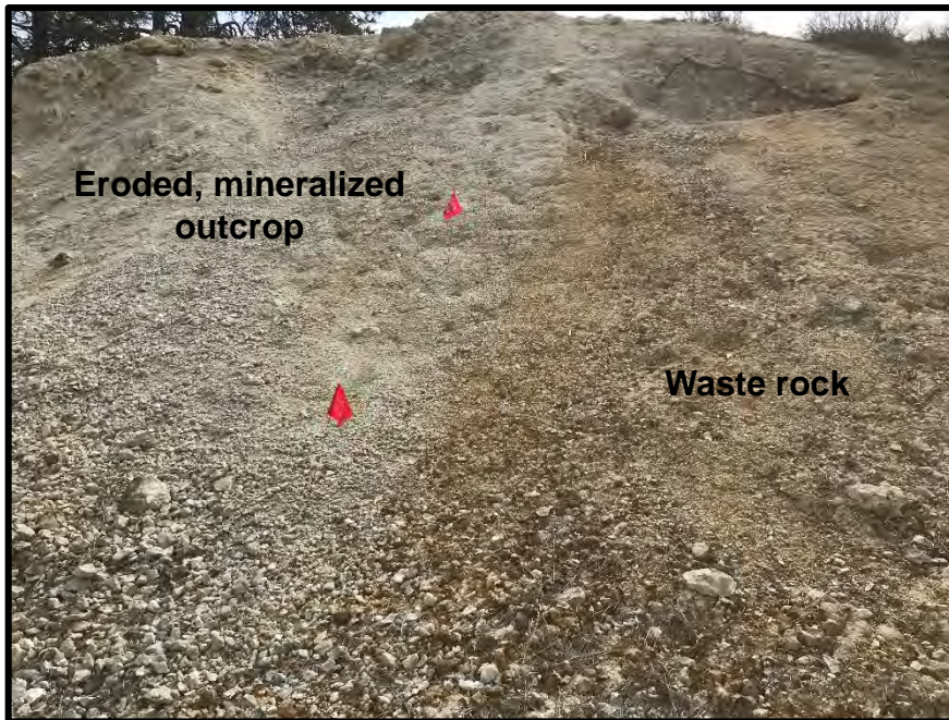
Photograph 29. Waste rock delineation at SR05. The waste pile limits were determined from observations and XRF confirmation. Eroded mineralized material to the left was not considered waste rock.
