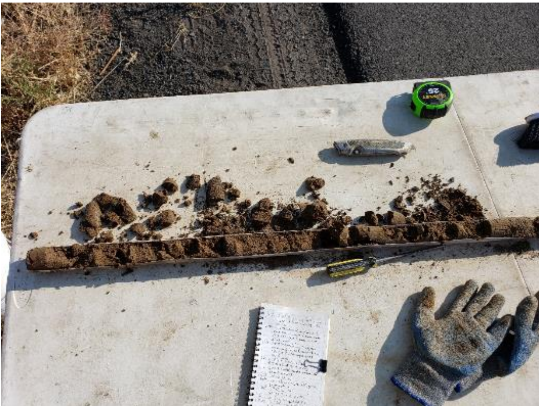
Photo 6. Soil cuttings from GP-4 at 0 to 4 feet. Soils in other borings at this depth interval are similar.
