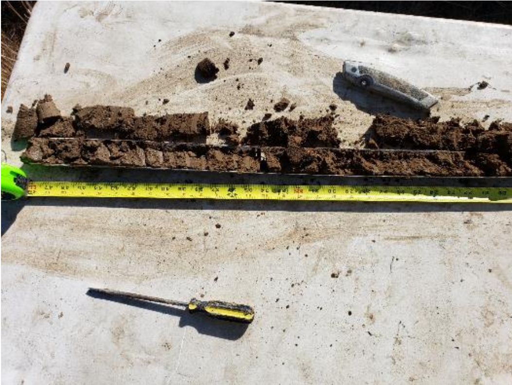
Photo 3. Soil cuttings from GP-1 at 0 to 4 feet. Soils in other borings at this depth interval are similar.
