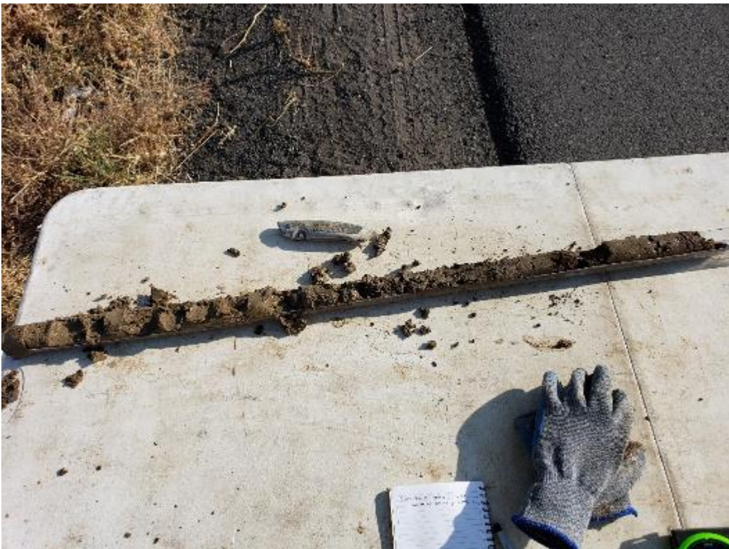
Photo 8. Soil cuttings from GP-4 at 8 to 12 feet. Soils in other borings at this depth interval are similar.
