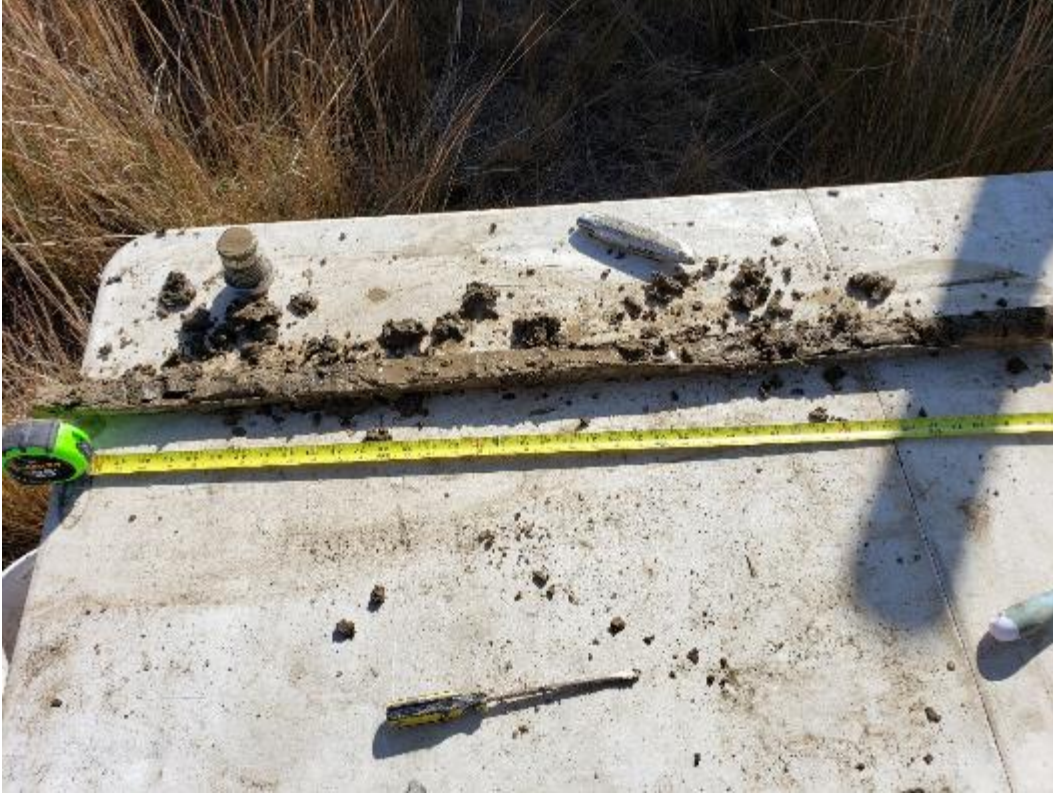
Photo 5. Soil cuttings from GP-1 at 8 to 12 feet. Soils in other borings at this depth interval are similar.
