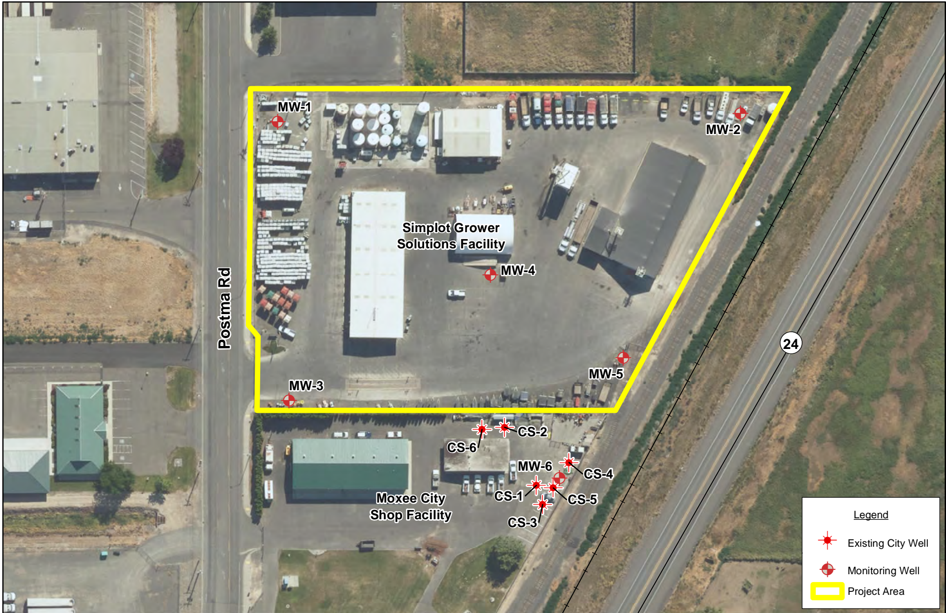
Figure 3. Existing Monitoring Well Network Simplot Grower Solutions, Moxee, WA
