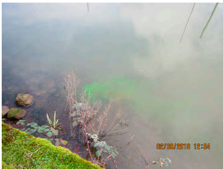
Photograph 6: Visual confirmation of dye discharging from CB-05 to the LDW via the South Park Marina outfall.
