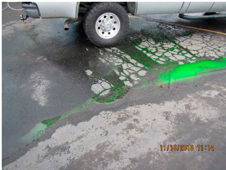
Photograph 10: Looking southeast at dye solution seeping up to ground surface through cracks in asphalt following the pumping of dye solution into the roof drain attached to the northeast corner of the RMM Shop.
