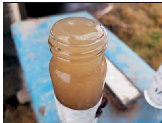
Grab Groundwater Sample Collected from AB5; Side View of the 40 ml VOA with the Observed Slight Sheen on the Meniscus
