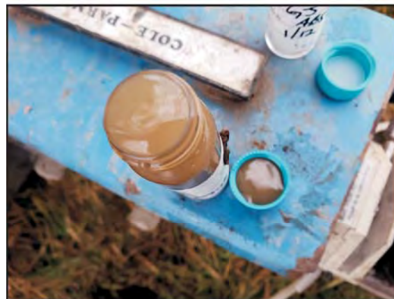
Grab Groundwater Sample Collected from AB5; Top View of 40 ml VOA with a Slight Sheen on the Meniscus
