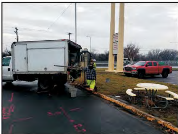
Heavy Duty Direct Push Drill Rig at Soil Boring Location AB5
