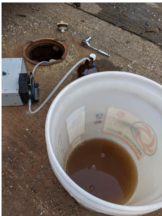
Photo 4. Groundwater sampling at SB-8. Some possible staining visible near well.
