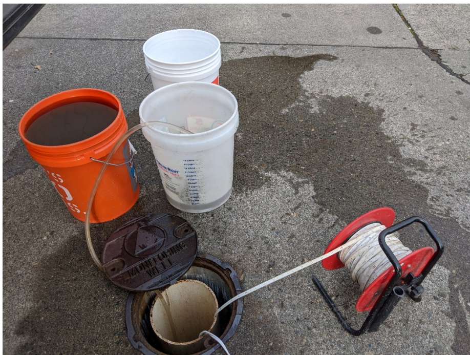
Photo 1. Turbid water being pumped out of well DW-4.
