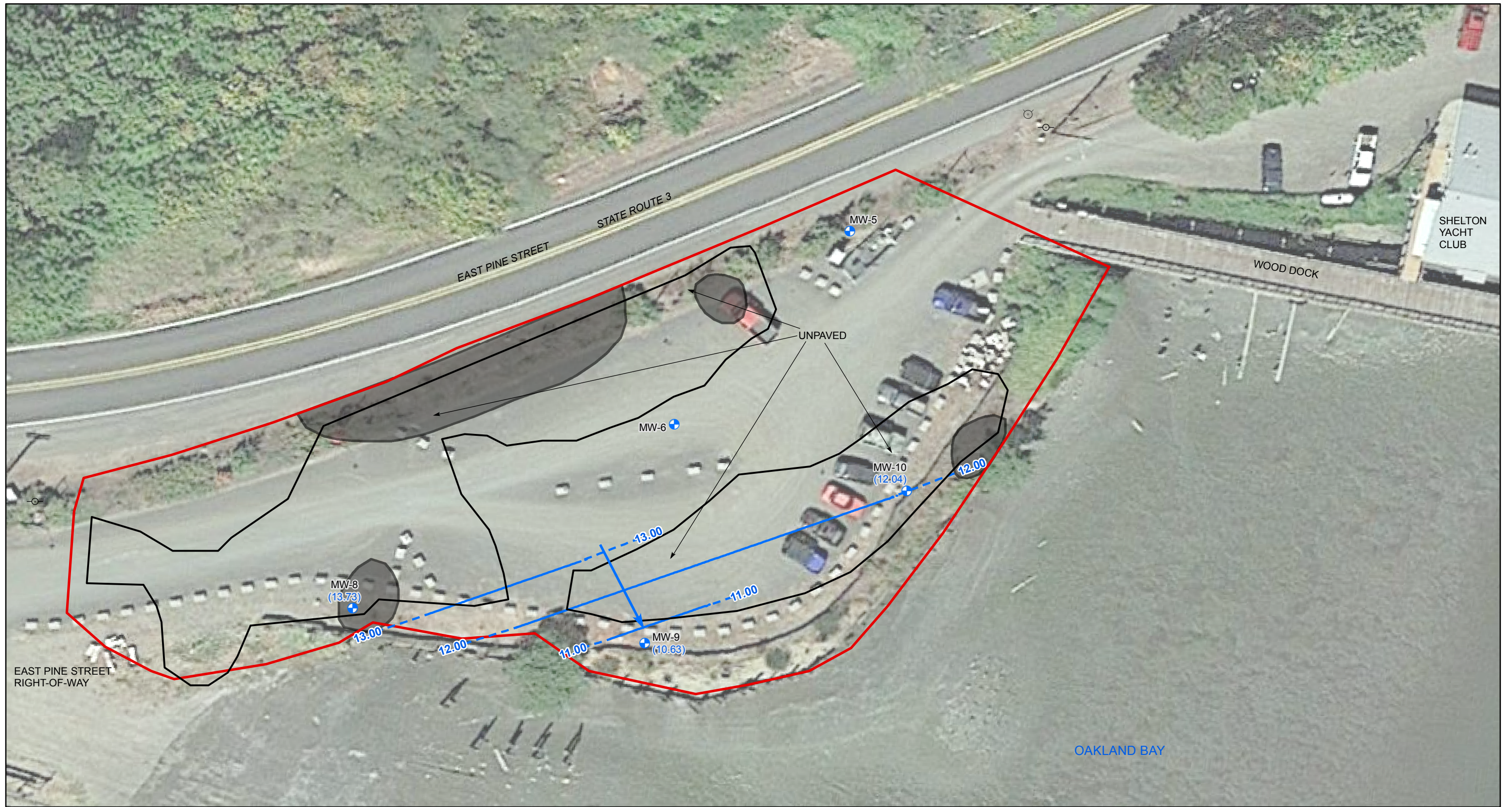
FIGURE 3 GROUNDWATER ELEVATION CONTOURS AND FLOW DIRECTION FEBRUARY 16, 2016 FORMER EVERGREEN FUEL FACILITY 661 EAST PINE STREET SHELTON, WASHINGTON FARALLON PN: 863-001
